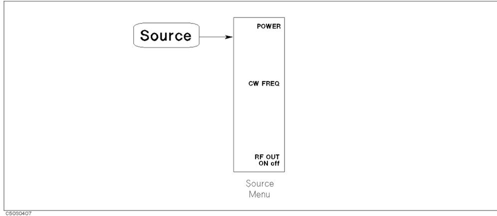
**Figure 4-8. Softkey Menus Accessed from the **Source** Key**
