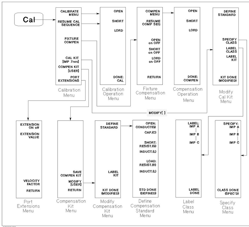
Figure 4-6. Softkey Menu Accessed from **Cal** key
