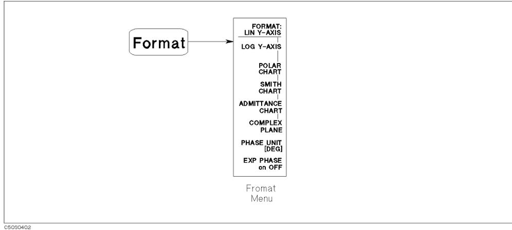
Figure 4-2. Softkey Menus Accessed from the **Format** Key
