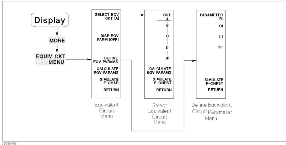
Figure 4-3. Softkey Menu Accessed from **Display** Key
